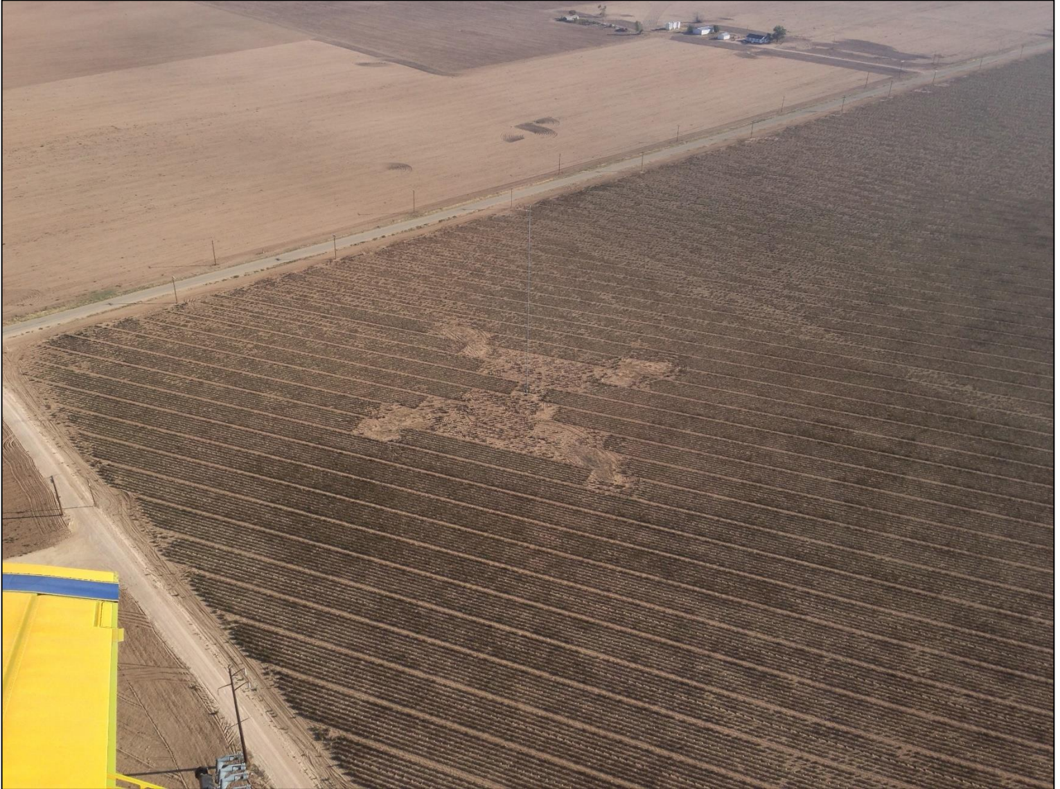
Figure 1: As this photograph taken in Texas in 2013 illustrates, unmarked towers are very difficult to see. This one taken from a pilot flying a low-altitude ag aircraft is only able to trigger further observation to search for a tower due to unmanicured soil surrounding the tower's footprint. Once the crop grows the footprint because harder to observe and sometimes farmers plant crops within the footprint making them more difficult to observe. Logging data should include the guy-wire footprint area surrounding the crop.
