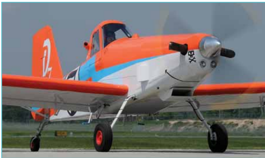
A live action version of Dusty Crophopper hit the air show circuit this summer flown by aerial applicator Rusty Lindeman of Rusty’s Flying Service, D’Hanis, Texas. Lindeman transformed his Air Tractor 301 into a turbine-powered AT-400A to go along with the Dusty paint scheme.
