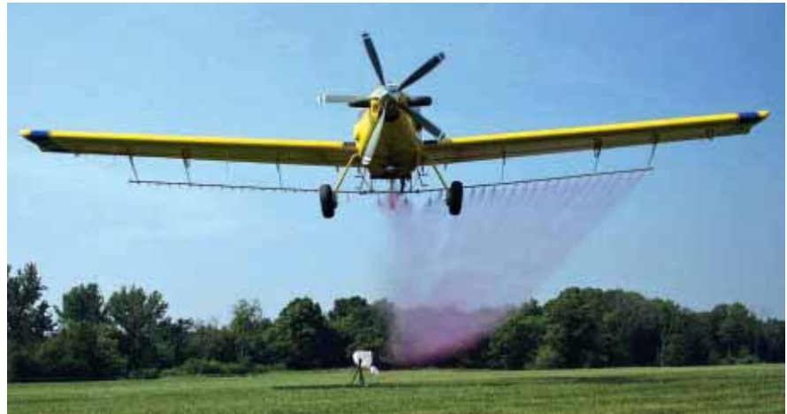
An aircraft makes a spray pass over the flight line with the right boom shut off at an Operation S.A.F.E. calibration clinic. The pink dye allows Operation S.A.F.E. analysts to analyze the spray pattern, determine the optimum swath width and make recommendations as needed to the pilot.
