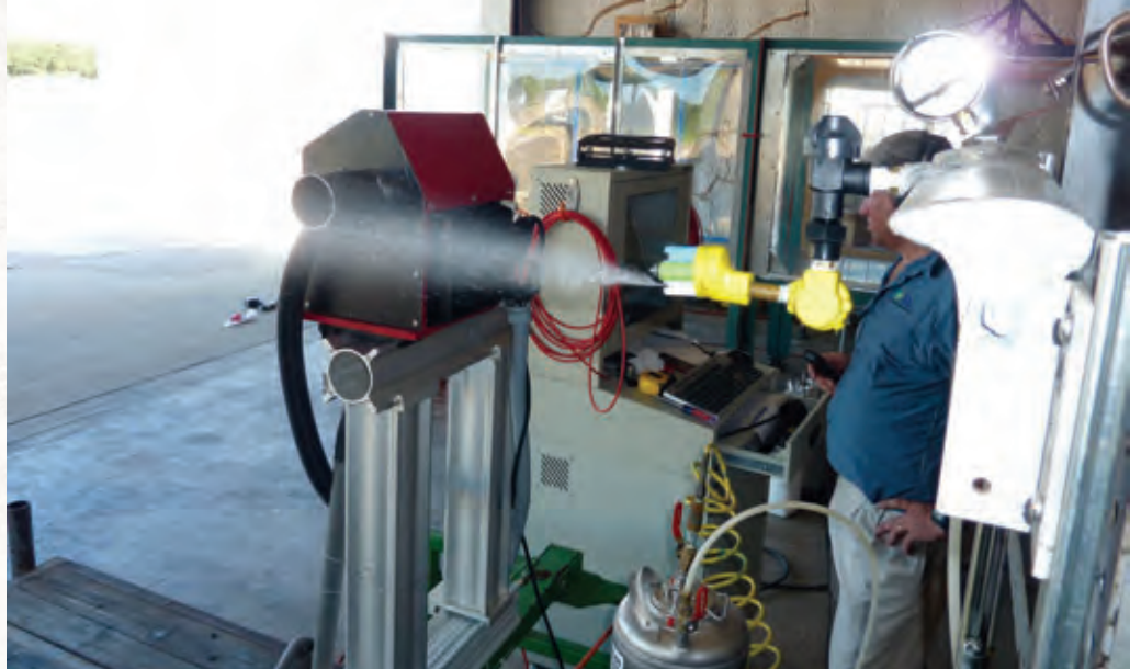
Testing nozzles in its high-speed wind tunnel is one of the ways the Aerial Application Technology group provides cutting-edge research for the aerial application industry.
