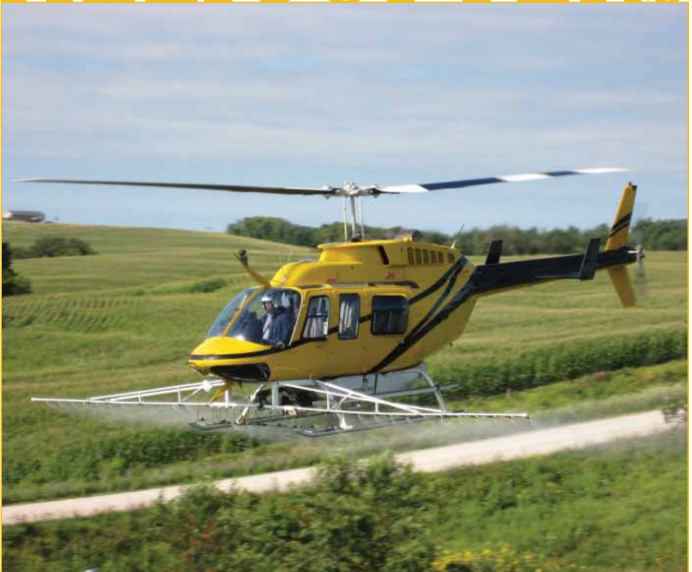
A Bell 206 LIII "Long Ranger" spraying BASF – Headline on soybeans in Iowa
