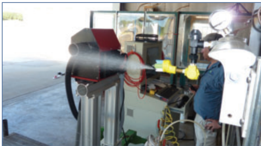
Spray nozzles are positioned at the outlet of the high speed wind tunnel, which can generate airspeeds up to 220 mph. The spray droplets are measured about 20 inches downstream with a laser droplet sizing instrument (red and silver instrument in the background).
