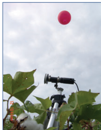
Sampling spray swath uniformity in cotton fields using cotton string. The balloon in the background is used to lift the string up out of the cotton so that it can be collected on reels for later analyses.
