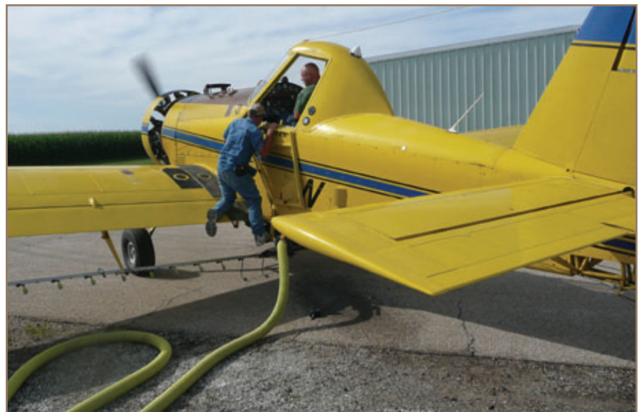
Hot fueling and loading in the aerial application industry involves both fueling and loading the hopper while the aircraft's engine is operating.
