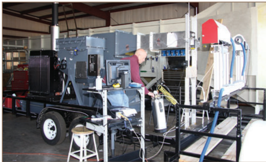
The Aerial Application Technology Group's new high speed wind tunnel and droplet sizing system is capable of airspeeds over 200 mph.
