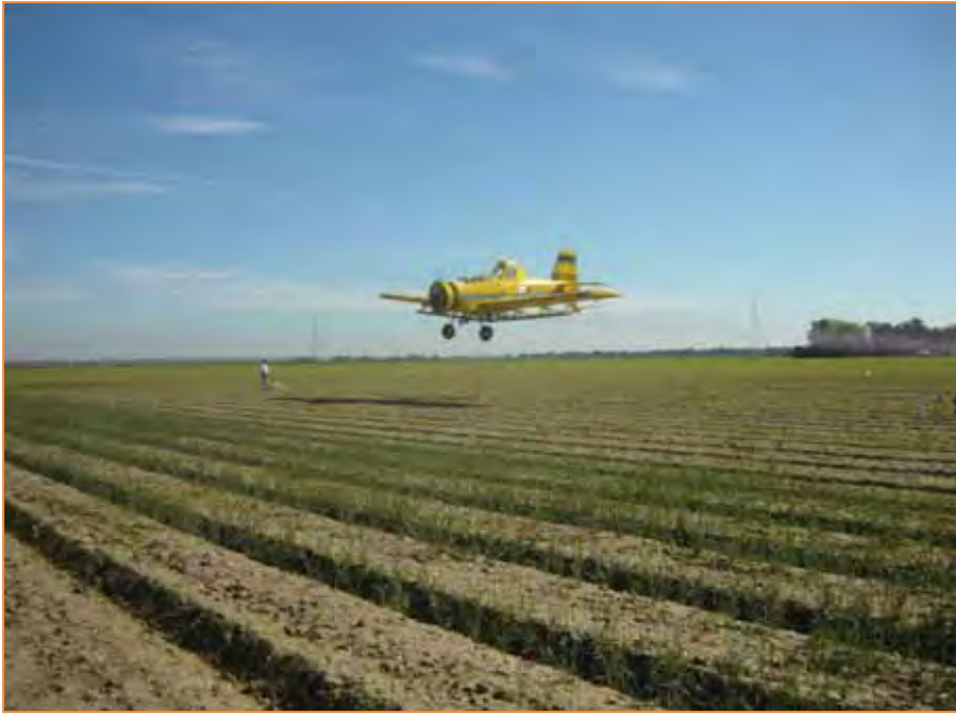
Figure 4. AT-301 with RVA chamber installed flying over the test plot.
