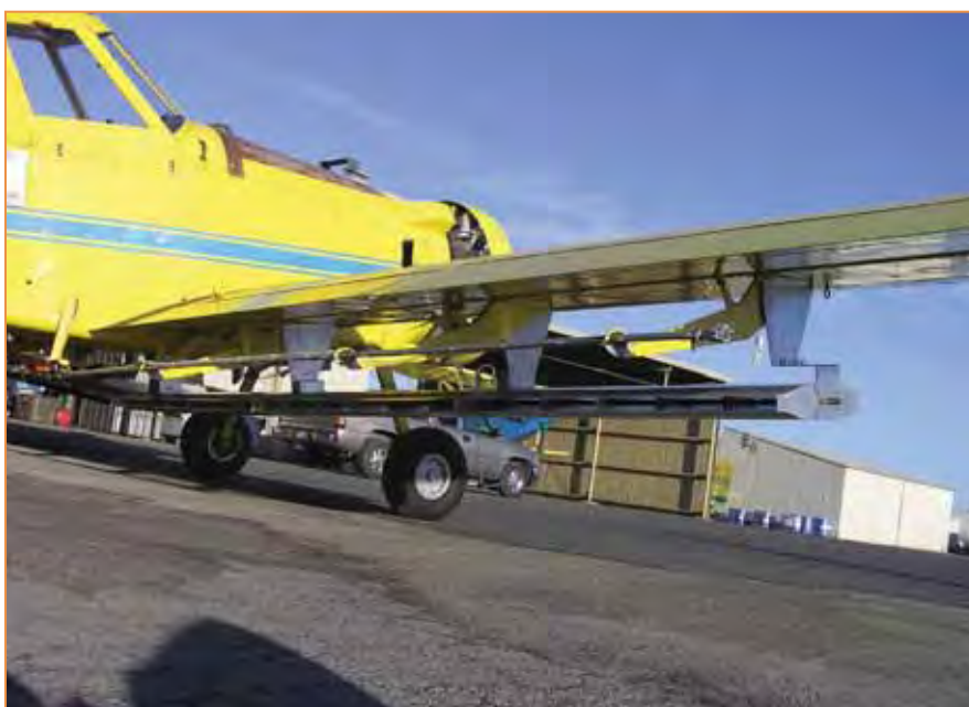
Figure 2. Full scale RVA Chamber installed on aircraft, two views. Note the conventional spray boom was maintained for testing.
