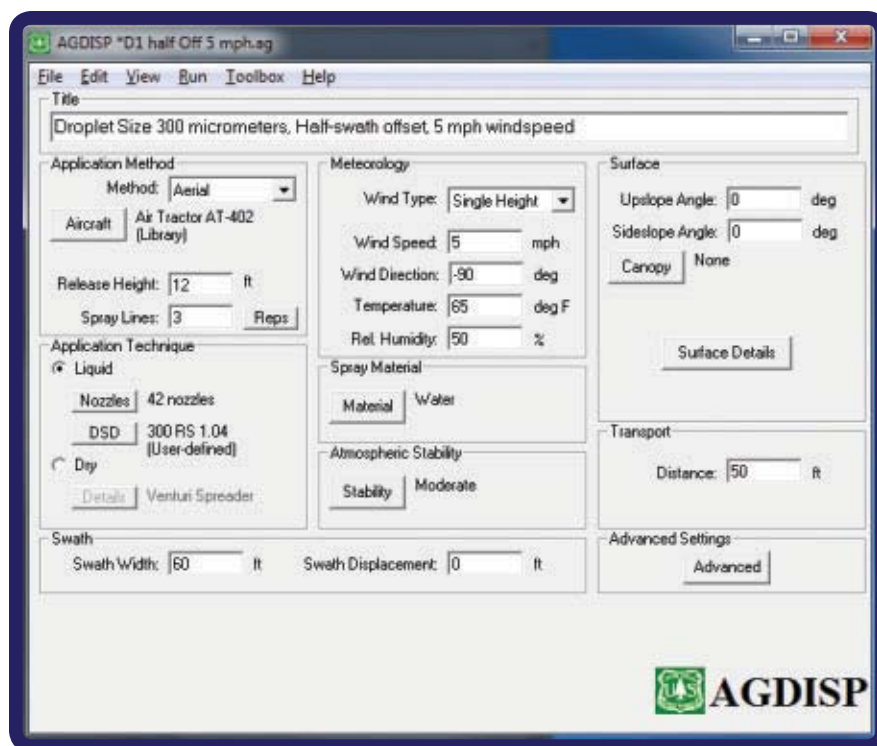
Fig. 1: Opening screen for the AGricultural DISPersion Model
