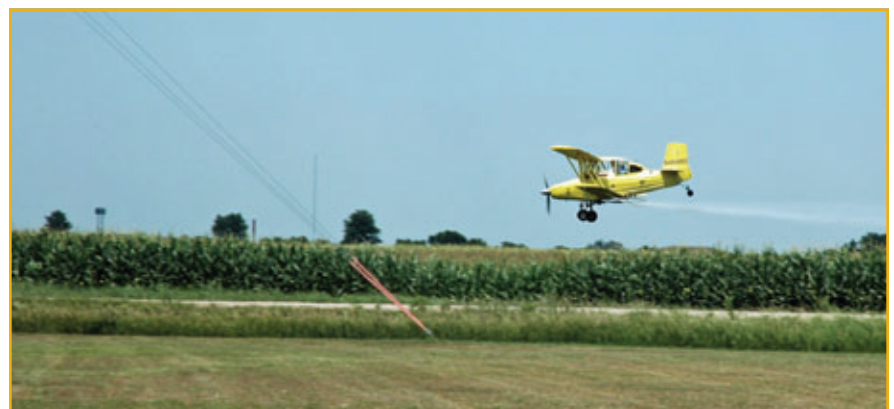
Obvious power lines are easy to see and avoid, but power lines and guy wires aren’t always in the places ag pilots would expect. They can even show up along the edge of a field.
