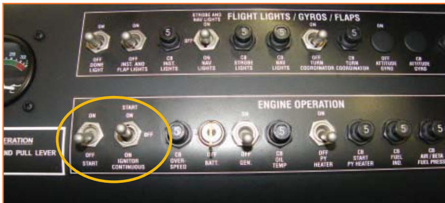
Example of an Air Tractor turbine panel showing the location of the “start” and “ignitor” switches on the left side of the engine operation panel.
