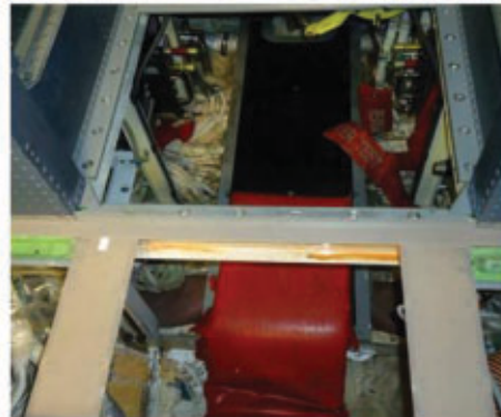
Structural tape installed directly to the structure of the aircraft.
