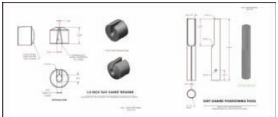
Diagram 3: Neoprene rubber retainer and the positioning tool to be attached to a pole.
