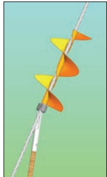
Diagram 1: The “Guy Guard” with its corkscrew design will spin in a breeze causing areas of reflected light, which appear to move lengthwise for high visibility. The illustration shows the rubber retainer below the marker and the installation pole with the positioning tool.
