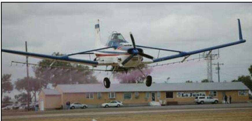
An airplane being pattern tested at the La Junta Operation S.A.F.E. Clinic.
